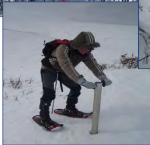
Taking a snow core to obtain snow density
