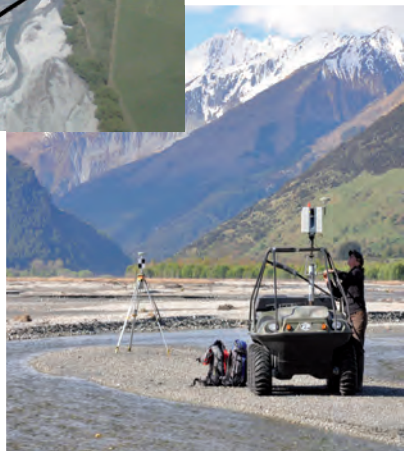
Images from my AGU poster: (above) the Rees River, New Zealand; (right) the ReesScan Terrestrial Laser Scanning system, mounted on an Argo All Terrain Vehicle.
